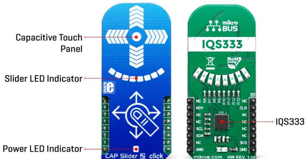
Capacitive touch sensing is based on detecting a change in capacitance, due to the influence of a foreign object. Basically, the capacitance of the sensor, also known as the
