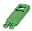
Strain relief for snapping into the latching chambers of the plug components, 4-pos., labeling with ZB 6
