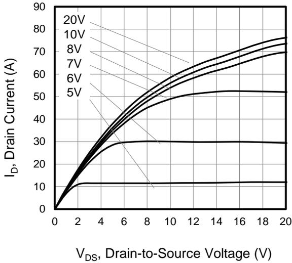
**Figure 1. Output Characteristics ( $T_J = 25^\circ\text{C}$ )**
