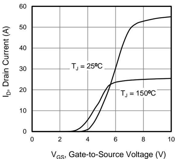
**Figure 5. Transfer Characteristics**
