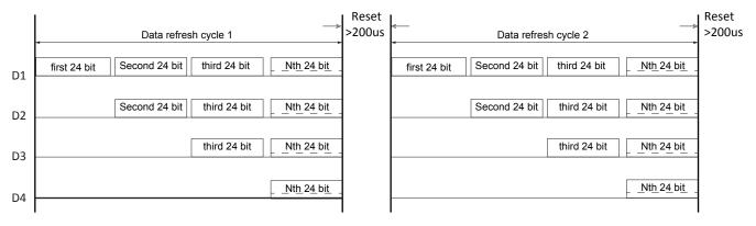
Note: Where D1 is the data sent by the MCU, D2, D3 and D4 are the data automatically shaped and forwarded by the cascade circuit.
