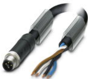
Power cable, 4-position, PUR halogen-free, black-gray RAL 7021, Plug straight M12, T-coded, on free cable end, cable length: 2 m, Customer version
