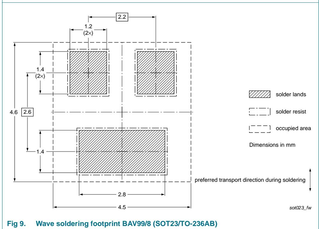
**Fig 9. Wave soldering footprint BAV99/8 (SOT23/TO-236AB)**
