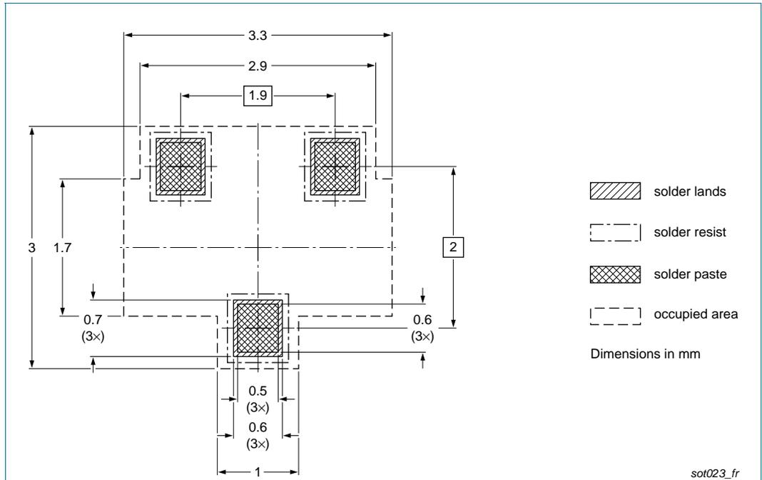
**Fig 8. Reflow soldering footprint BAV99/8 (SOT23/TO-236AB)**
