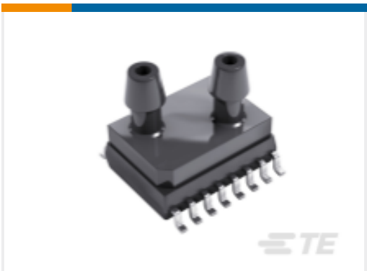
TE Part #9541-100C-D-C-3-S PRESSURE I2C 1.5 PSID SO16
