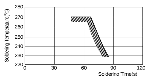
[Allowable Reflow Soldering Temperature and Time]
