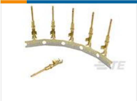
TE Part #1060-20-0244 PIN, SF, SIZE 20, 16-22, AU/SN
