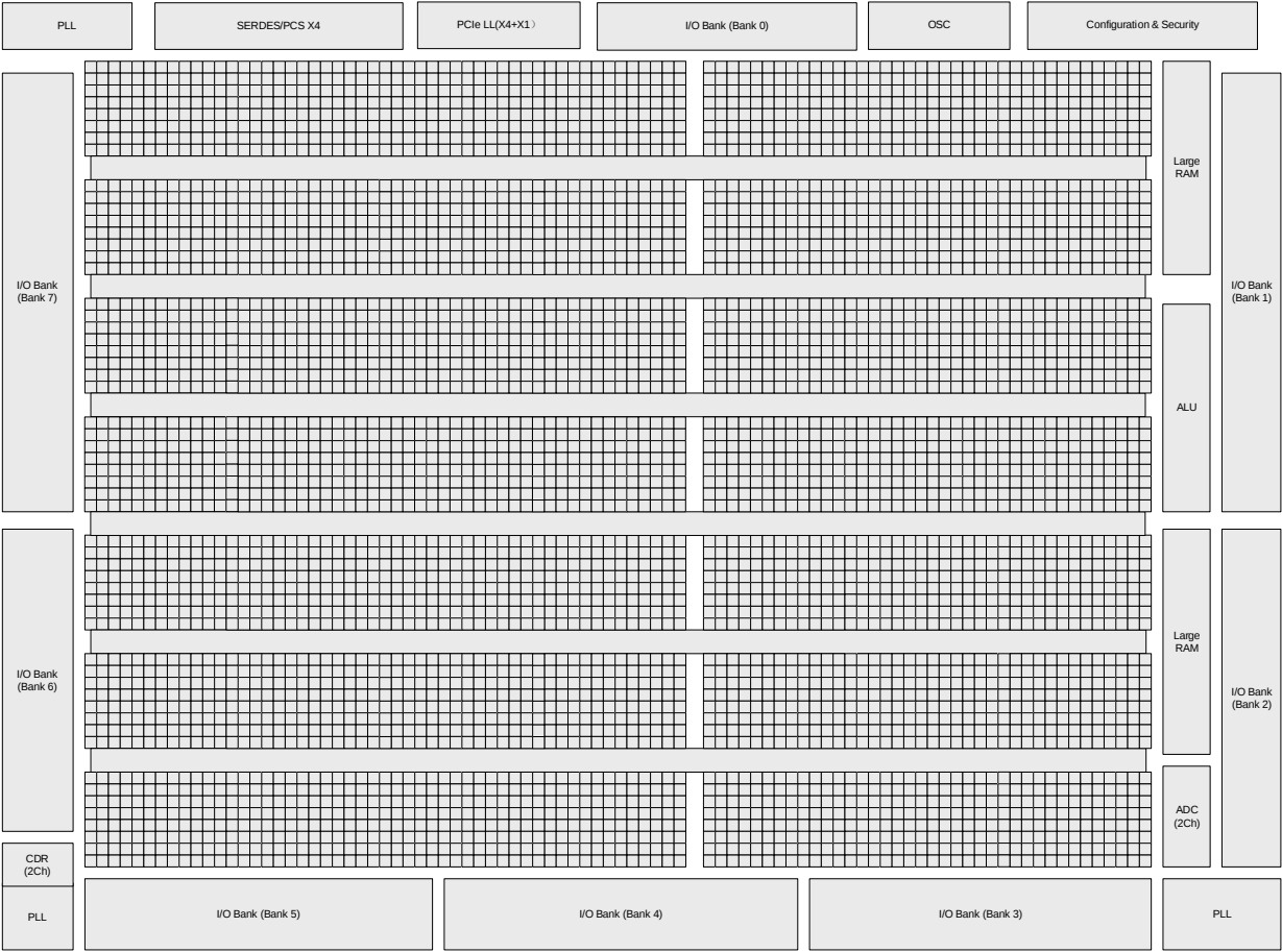
Figure 2.1. Simplified Block Diagram, LFCPNX-50 Device (Top Level)
