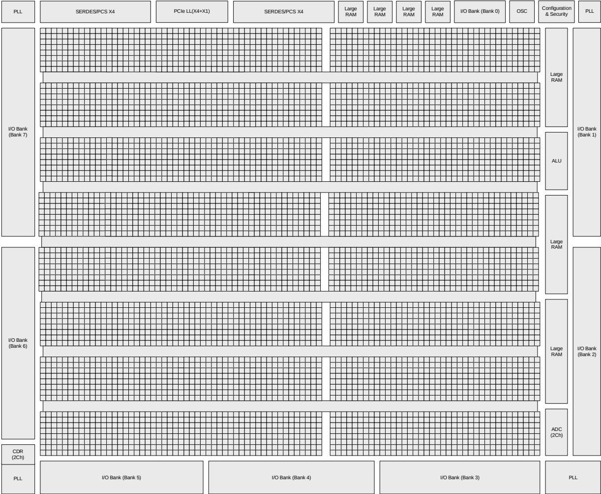
Figure 2.2. Simplified Block Diagram, LFCPNX-100 Device (Top Level)
