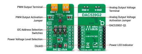
What sets DAC 18 Click apart is its nonvolatile memory (NVM) capability, which allows users to store customized register settings during programming via I2C. Once configured, the device can function independently, executing the predefined instructions. This feature makes it ideal for applications such as fault communication in automotive stop-and-turn lighting systems and broader industrial environments where reliable signal conversion is essential.
