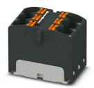
Distribution block, bridged internally, nom. voltage: 450 V, nominal current: 32 A, number of connections: 6, connection method: Push-in connection, cross section: 0.2 mm² - 6 mm², mounting type: for snapping onto a DIN rail adapter, Direct mounting with flange, Free-hanging, color: black
