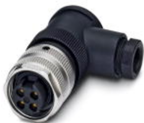
Connector, Universal, 4-position, Socket angled 7/8"-UNF, A-coded, Screw connection, knurl material: Zinc die-cast, nickel-plated, cable gland Pg9, external cable diameter 6 mm ... 8 mm
