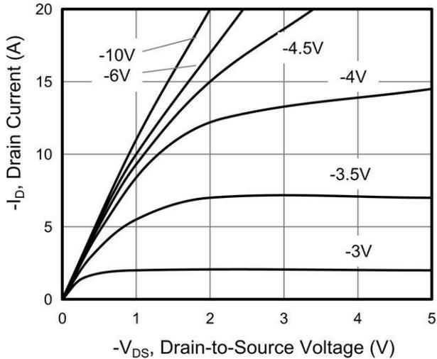
Figure 2. Transfer Characteristics
