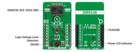
Diff Press 4 Click can use a standard 2-wire I2C interface to communicate with the host MCU, where you can read both the pressure and the temperature measurements. As the SM9336-BCE-S-250-000 sensor works on 3.3V, this Click board™ comes equipped with the PCA9306, a dual bidirectional I2C bus and SMBus voltage-level translator from Texas Instruments, which allows the use of this Click board™ with systems with 5V logic level.
