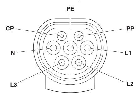
Pin assignment of the Vehicle Connector
