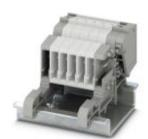
COMBI receptacle, Connection method: Push-in connection, Number of positions: 9, Cross section: 0.14 mm² - 1.5 mm², AWG: 26 - 14, Width: 31.5 mm, Height: 27.1 mm, Color: gray, Mounting type: NS 35/15, NS 35/7,5
