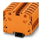
High-current terminal block, nom. voltage: 1000 V, nominal current: 125 A, number of connections: 2, number of positions: 1, connection method: PowerTurn connection, Rated cross section: 35 mm<sup>2</sup>, cross section: 2.5 mm<sup>2</sup> - 35 mm<sup>2</sup>, mounting type: NS 35/15, color: orange
