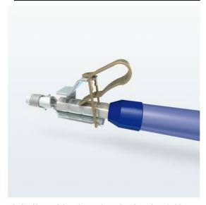
Whether it's a push-in spring or a leg spring, the spring principle makes for quick, tool-free conductor connection. Simply insert the solid conductors and conductors with ferrules into the push-in terminal point and release using a screwdriver. When connecting and releasing finely stranded conductors without ferrules, the terminal point can also be opened using a screwdriver.
