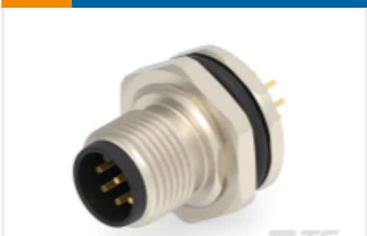
TE Part #T4140012081-000 M12,REAR MOUNT,MALE,A,8P, SOLDER PCB
