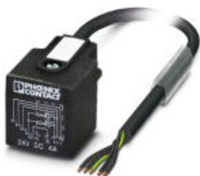
Sensor/actuator cable, 5-position, PUR halogen-free, black-gray RAL 7021, free cable end, on Valve connector AD (pressure switch), with 2 LEDs, cable length: 5 m
