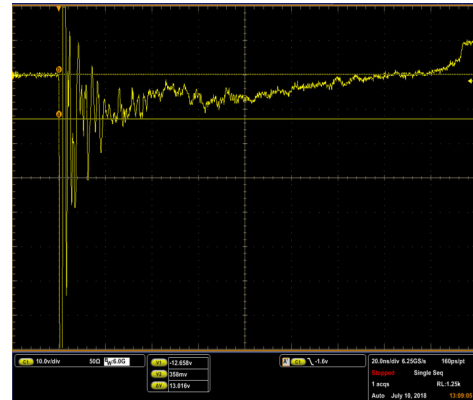
IEC 61000-4-2 -8 kV Contact ESD Clamping Voltage
