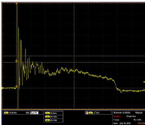
IEC 61000-4-2 +8 kV Contact ESD Clamping Voltage
