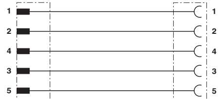
Contact assignment of the M12 plug and the M12 socket
