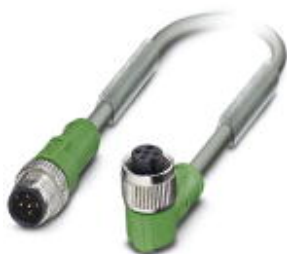
Sensor/actuator cable, 5-position, PUR halogen-free, welding sputter-resistant, highly flexible, gray RAL 7001, Plug straight M12, A-coded, on Socket angled M12, A-coded, cable length: 5 m
