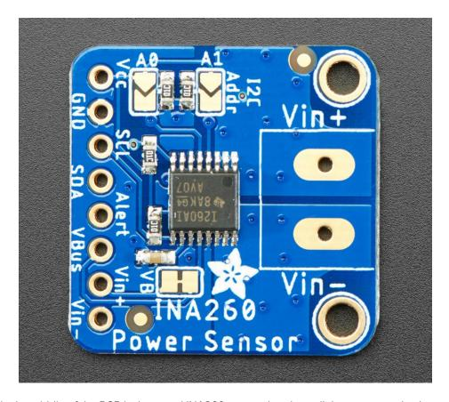
The little chip in the middle of the PCB is the actual INA260 sensor that does all the current and voltage sensing. We add all the extra components you need to get started, and 'break out' all the other pins you may want to connect to onto the PCB. For more details you can check out the schematics in the Downloads page.
