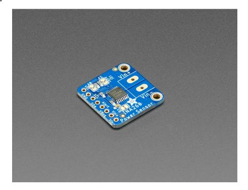
This breakout board may well be the last current sensing solution you every need to buy. Not only can it do the work of two multimeters, but it can do it with amazing precision and flexibility. With it you can measure high or low side DC current, the bus voltage, and have it automatically calculate the power. It can do so over impressive voltage, current, and temperature ranges with better than 1% accuracy, all while delivering the data in an easy to use format over I2C.
