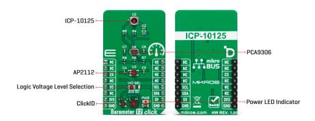
Barometer 12 Click uses a standard 2-Wire I2C interface to communicate with the host MCU supporting clock frequency up to 400KHz. To allow safe sensor operation on both 5V and 3.3V voltage logic, this Click board  $^{\text{\tiny M}}$  features the PCA9306, a dual bidirectional I2C bus and SMBus voltage-level translator from Texas Instruments.
