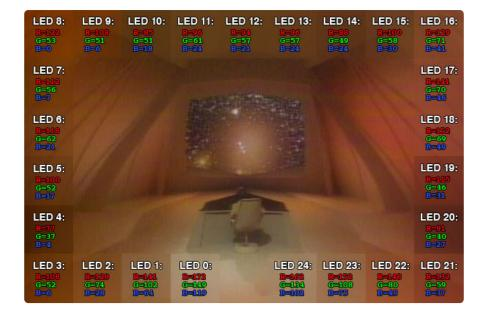
If you plan to arrange the LEDs similarly to our examples — 25 pixels in a ring, 1 pixel gap at the bottom, with the first pixel starting just left of the gap — then nothing more needs to be changed in the software. If using a different layout, you'll need to make adjustments in the code. You'll find extensive notes in the source code for making this (and other) changes.
