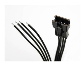
Alternately, if you don't want to use the "jammed wires" trick, an optional mating connector is available in the Adafruit shop (http://adafru.it/579). This has a plug housing at one end and four tinned wires at the opposite end...strip a little more insulation to press these into Arduino pin sockets.
