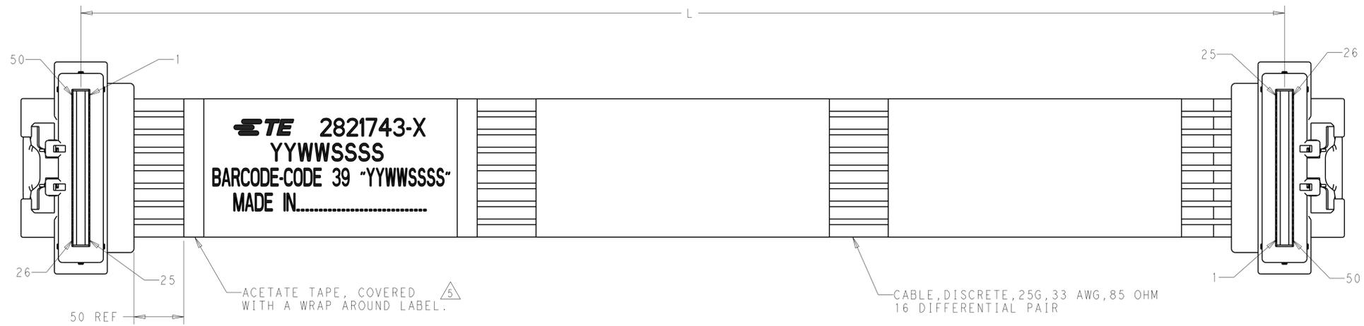
1. CABLE ASSEMBLY TO BE TESTED FOR OPENS, SHORTS AND WIRING MAPPING. CABLES ARE ALSO TO BE TESTED FOR SIGNAL INTEGRITY. 10% OF PRODUCT TO BE TESTED FOR SIGNAL INTEGRITY.
