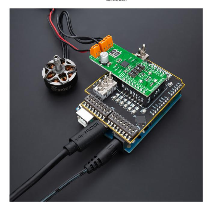
When the USB Type C connector is connected to the Protolino Click Shield, and the other USB is connected to the Arduino Uno Rev3 board, the PWR diode will glow Cyan, and at this setup, the mikroBUS™ socket is powered from the Type C connector. The Arduino Uno Rev3 board is unloaded from delivering power to them and is powered from its source (Arduino's USB), over which you can also upload the program to your board.
