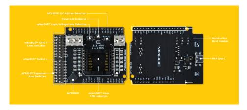
Protolino Click Shield is an adapter board for the Arduino family, precisely for the Arduino Uno Rev3 board, with only one onboard mikroBUS™ socket. This way, Mikroe allows its users to add any functionality from our ever-growing range of Click boards™, such as WiFi, GSM, GPS, Bluetooth, ZigBee, environmental sensors, LEDs, speech recognition, motor control, movement sensors, and many more.
