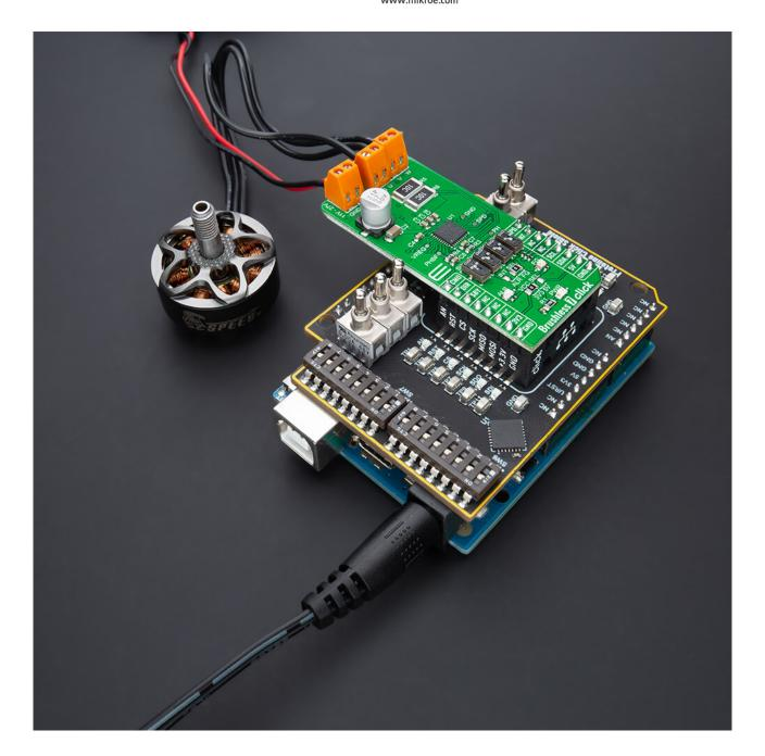
When the USB is connected to the Arduino Uno Rev3 board, the PWR diode will glow Green, and at this setup, the Arduino baseboard itself will be powered and will provide power to the Protolino Click Shield, including mikroBUS™ socket.
