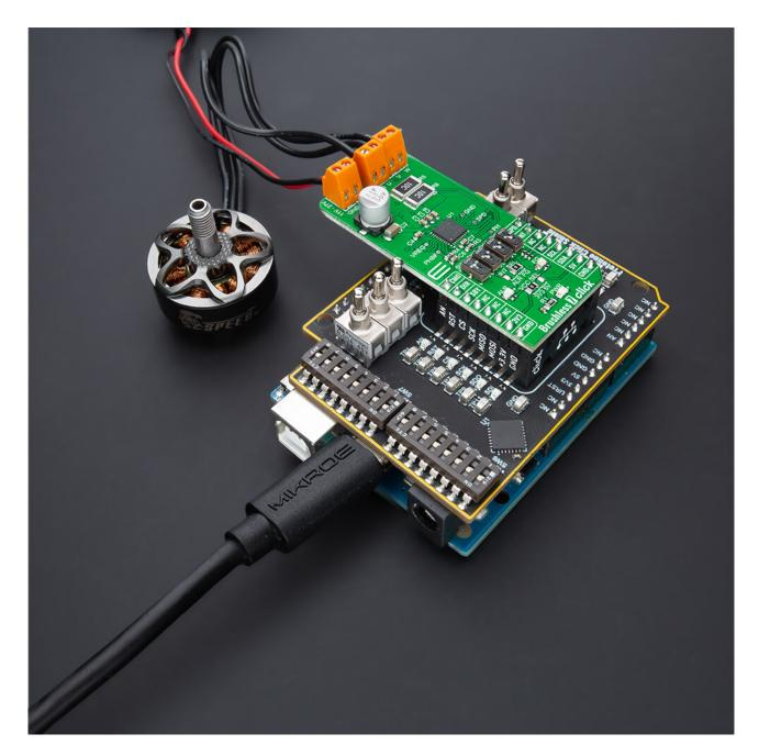
When the USB type C connector is connected to the Protolino Click Shield, the PWR diode will glow Blue, and at this setup, the connected Arduino Uno Rev3 baseboard and mikroBUS™ socket will be powered from it.
