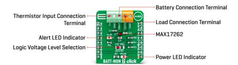
The ModelGauge™ m5 EZ algorithm combines the short-term accuracy and linearity of a Coulomb counter with the long-term stability of a voltage-based fuel gauge, along with temperature compensation, to provide industry-leading fuel-gauge accuracy. The MAX17262 automatically compensates for cell aging, temperature, and discharge rate, providing accurate state-of-charge in percentage (%) and remaining capacity in milliampere-hours (mAh) over a wide range of operating conditions.
