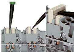
**Removing a push-in type jumper bar:** Insert the operating tool between the jumper and partition wall of the dual jumper slots, then lift up the jumper. Place the operating tool in the center of jumpers for up to five contacts (see above), or alternately on both sides for jumpers with more than five contacts.
