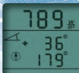
Insolation, angle of inclination and compass bearing
