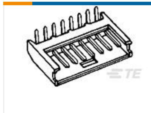
TE Part #280379-2 6P MODU II SHRD HDR, RT ANG, 0.38 AU
