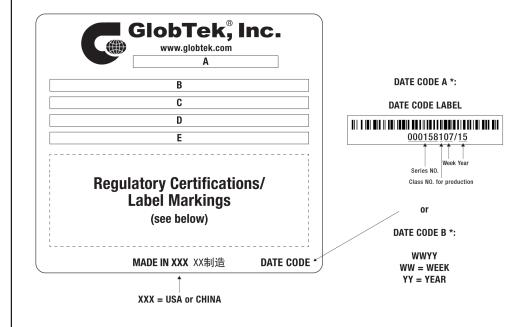
A=Medical/ICT/ITE/Household use Power Supply B=P/N: (料号) TR9CE13330A04CIMR6B C=Model (型号) GTM961800P16012-T3 D=Input (输入)100-240V~, 50-60Hz, 2.2A E=Output (输出)12.0 V === 13.33 A, 160.00W
