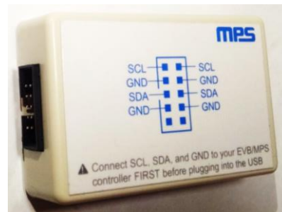
Figure 3: EVKT-USBI2C-02 Communication Interface
