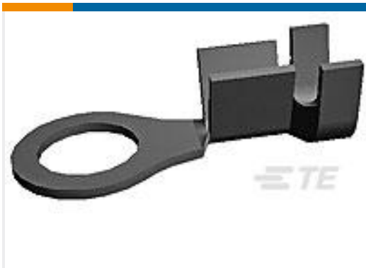
TE Part #40955 RING 20-16 AWG .0295 X .390 TPBR
