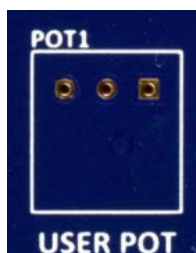
Figure 26. User Potentiometer on Target Board (Top)
