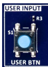
Figure 16. User Switch (S1) on Target Board
