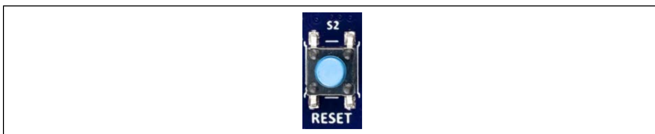
Figure 18. Reset Switch (S2) on Target Board
