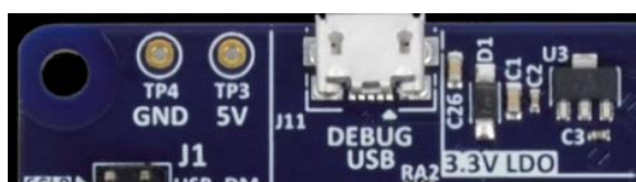
Figure 6. USB Debug Connector (J11), TP3, and TP4 on Target Board
