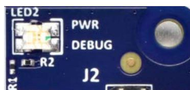
Figure 10. LED2 on Target Board (Top Side)
