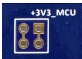
Figure 13. E6 on Target Board (Bottom Side)
