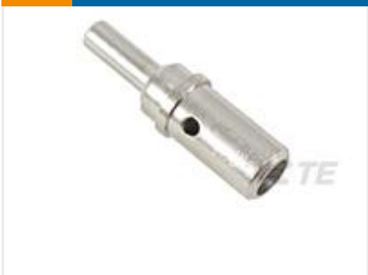
TE Part #0460-204-08141 PIN, SOLID, SIZE 8, 8-10AWG, NI
