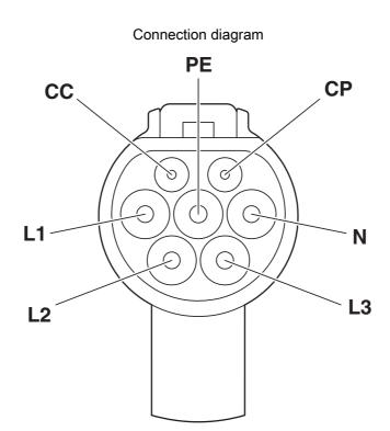
Pin assignment of the Vehicle Connector
