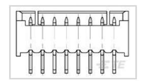
PCB Connector Assembly Type: PCB Mount Header
