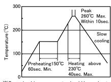
%Ceramic chip components should be preheated to within 100 to 130°C of the soldering.
