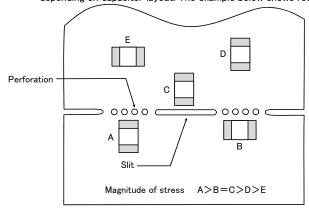
1-3. When breaking PC boards along their perforations, the amount of mechanical stress on the capacitors can vary according to the method used. The following methods are listed in order from least stressful to most stressful: push-back, slit, V-grooving, and perforation. Thus, any ideal SMD capacitor layout must also consider the PCB splitting procedure.
