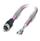
Bus system cable, CANopen®, DeviceNet $^{\text{TM}}$ , 5-position, PUR halogen-free, red lilac RAL 4001, shielded, free cable end, on Socket straight M12, coding: A, cable length: 15 m
