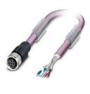
Bus system cable, CANopen®, DeviceNet™, 5-position, PUR halogen-free, red lilac RAL 4001, shielded, free cable end, on Socket straight M12, coding: A, cable length: 5 m
