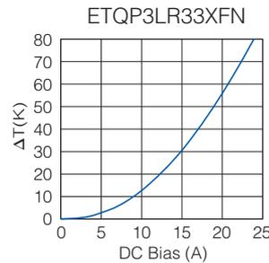
PWB condition A : FR4, single layer PWB, t=1.6mm \*our specification
