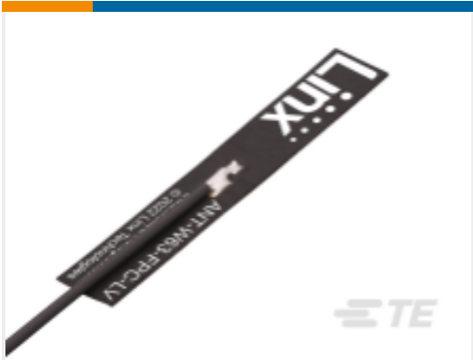
TE Part #L9000211-01 Antenna WiFi6/6E FPC LV 7x45 100 UFL
