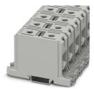
High-current terminal block, nom. voltage: 1000 V, nominal current: 220 A, number of connections: 2, number of positions: 1, connection method: Screw connection, Rated cross section: 95 mm<sup>2</sup>, cross section: 16 mm<sup>2</sup> - 95 mm<sup>2</sup>, Rated cross section: 95 mm<sup>2</sup>, cross section: 16 mm<sup>2</sup> - 95 mm<sup>2</sup>, mounting type: NS 35/15, NS 35/7,5, color: gray
