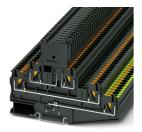
Fuse modular terminal block, fuse type: Glass / ceramics / ..., fuse type: G / 5 x 20, nom. voltage: 24 V, nominal current: 6.3 A, connection method: Push-in connection, Rated cross section: 4  $\text{mm}^2$ , cross section: 0.2  $\text{mm}^2$ - 6  $\text{mm}^2$ , connection method: Push-in connection, cross section: 0. 2  $\text{mm}^2$ - 6  $\text{mm}^2$ , mounting type: NS 35/7,5, NS 35/15, color: black
