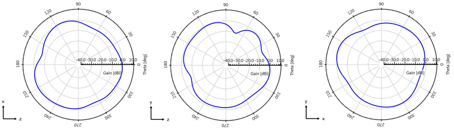
**Band 4 Rx measured at 2110 MHz**
