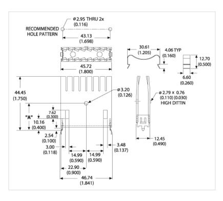
X Dim: 21.56 (0.849) | Y Dim: 6.35 (0.250) | YT Dim: 12.70 (0.500) | Z Dim: 2.95 (0.116)
