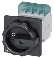
SENTRON, Switch disconnector 3LD, main switch, 4-pole, lu: 16 A, Operating power / at AC-23 A at 400 V: 7.5 kW, front-mounted, rotary operating mechanism, black, central mounting 22.5 mm of the handle
