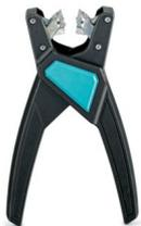
Stripping pliers, for halogen-free sensor/actuator cables (SAC cables), with PUR and PVC insulation, from Ø of 4.4 to 7 mm, any stripping length
