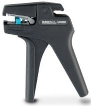
Stripping tool, for conductors and cables with a conductor cross section from 0.08 to 2.5 mm, self-adjusting, stripping length adjustable up to 15 mm, cutting capacity up to 6 mm<sup>2</sup> stranded/1.5 mm<sup>2</sup> solid
