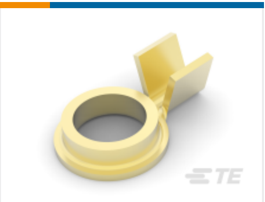
TE Part #160088-3 RING TONGUE 20-16 AWG 0.198 X . 700 BR
